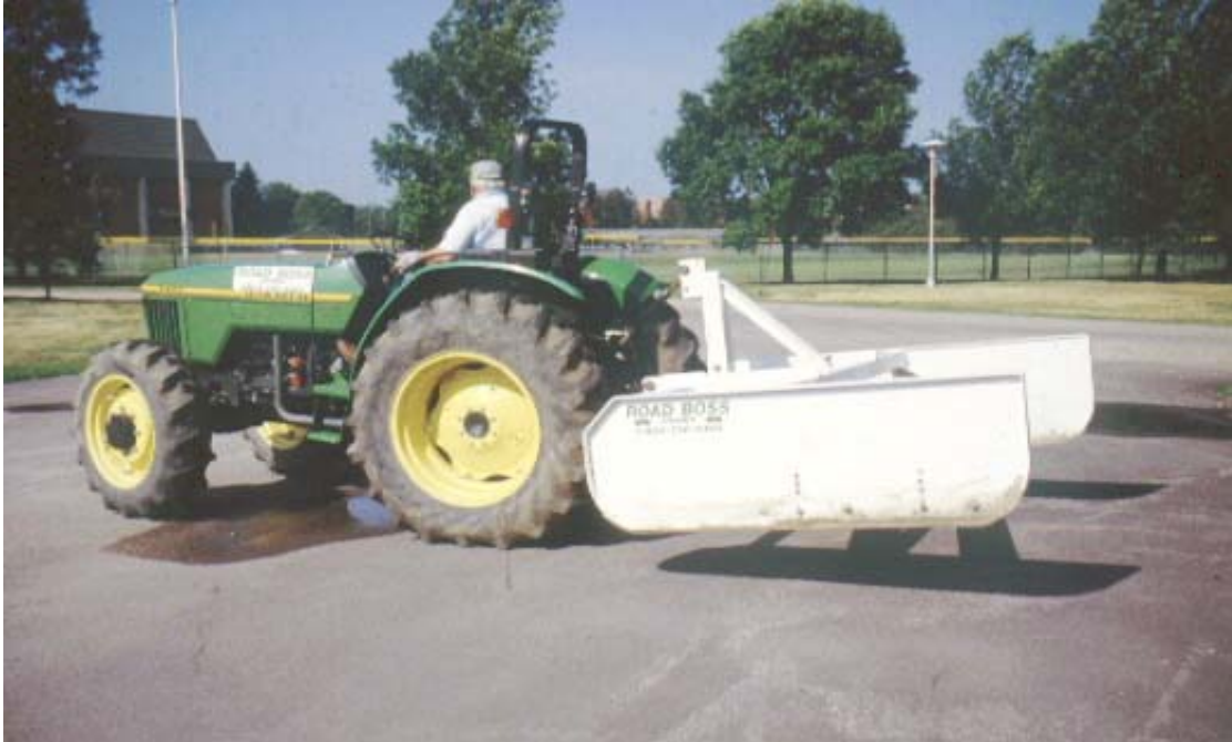
Figure 7: A removable rear-mounted blading attachment on a tractor
